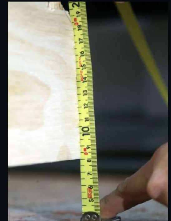
Measurements of internal unevenness of the building's floor.
